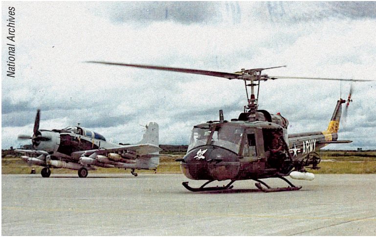
A UH-1 Huey gunship idles on an airfield next to an A-1 Skyraider attack aircraft.
